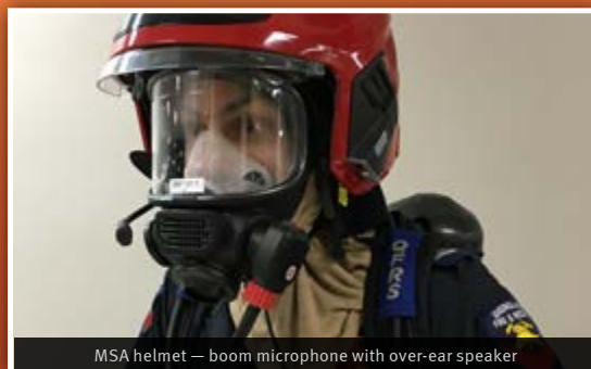
MSA helmet — boom microphone with over-ear speaker
