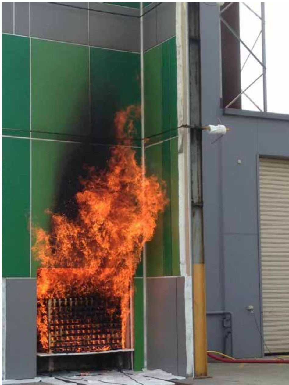
Aluminium Composite Panels undergoing testing.
