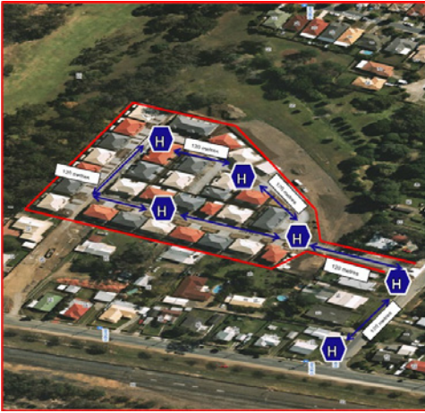
Figure 6 – Hydrant System design to minimum standards
