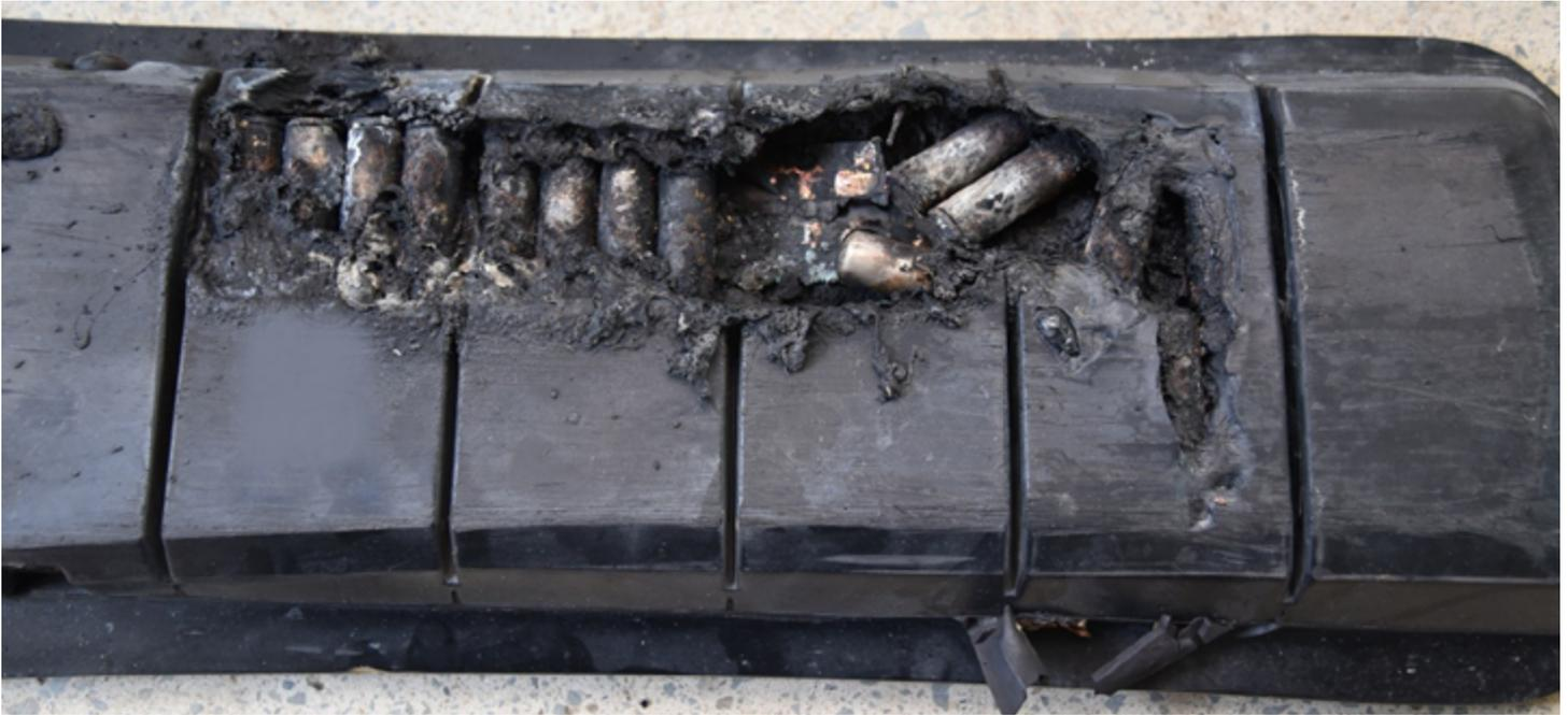
Batteries inside an electric skateboard displayed extensive blowout.
