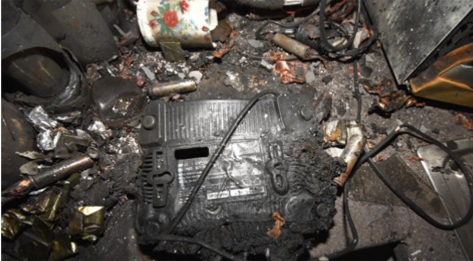
*A lawnmower battery exploded being on charge and unattended to for 35 hours.*
